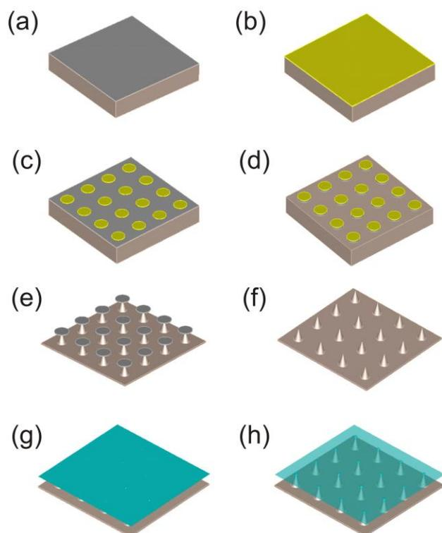
Figure 1: Schematic of the processes of transferring the CVD graphene onto the Mo tip array: (a) deposition of 300nm Al, (b-c) photoresist patterning by optical lithography, (d) ICP etching of Al, (e) Mo tip forming ICP etch, (f) removal of Al mask, (g) PMMA/graphene film transfer, and (7) PMMA removal by heating.
