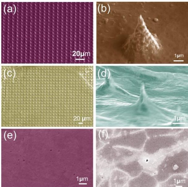
Figure 3: SEM of (a) Mo tip arrays (b) Perspective view of single Mo tip (c) Mo tip arrays with graphene (d) Perspective view (e) Bulk Mo (f) Bulk Mo with graphene.
