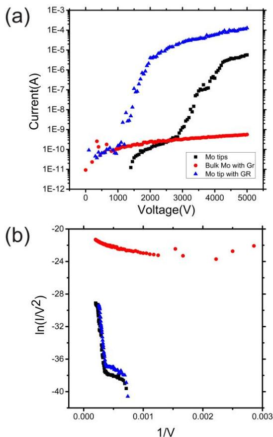
Figure 5: I-V curves of Mo tips, Bulk Mo/graphene and Mo tips/graphene cathodes. (b) Corresponding FN plots.
