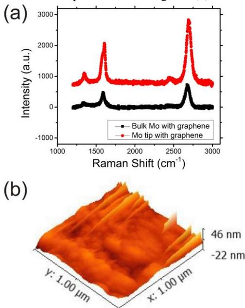
Figure 4: (a) Raman shift of bulk Mo/graphene and Mo tips/graphene (b) Surface roughness of the graphene on the Mo tips.
